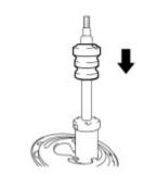
(a) Install the front spring bumper to the front shock absorber assembly.
