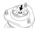
(b) Temporarily tighten a new front support to front shock absorber nut.
