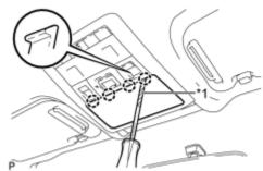
(1) Using a screwdriver with its tip wrapped with protective tape, disengage the 4 claws and disconnect the cover.
