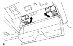
(3) Rotate the 2 caps as shown in the illustration until the screws are visible.
