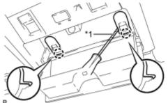
(2) Using a screwdriver with its tip wrapped with protective tape, disengage the 2 claws.
