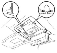
(b) Engage the 2 clips and 2 claws, and install the map light assembly.
