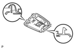
(b) Engage the 4 claws and install the No. 1 room light housing.
