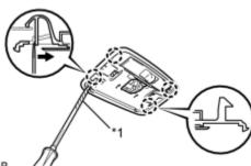
(c) Using a screwdriver with its tip wrapped with protective tape, disengage the 4 claws and disconnect the No. 1 room light housing as shown in the illustration.
