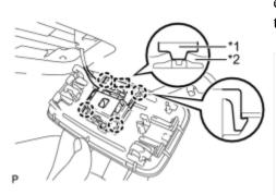
(a) Align the switch parts shown in the illustration and engage the 4 claws to install the room light switch base to the No. 1 room light housing.
