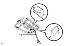
(b) Using a screwdriver with its tip wrapped with protective tape, disengage the 2 claws and 2 guides, and remove the 2 No. 1 room light covers.
