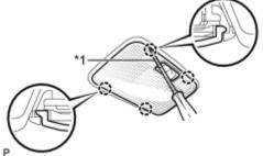
(a) Using a screwdriver with its tip wrapped with protective tape, disengage the 4 claws and remove the No. 1 room light lens.
