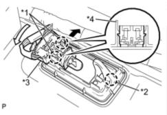
(a) Tilt the tab to disengage the 2 claws <A> and separate the bulb holder from the vanity light as shown in the illustration.
