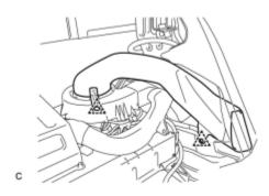
(a) Remove the 2 clips and No. 1 HV battery intake duct.
