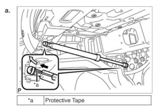
Use a thin-bladed flat-head screwdriver wrapped in protective tape to remove the two stop rings along the grooves.
