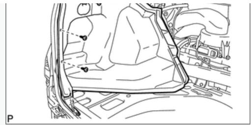
13.Remove rear combination lamp socket & wire SUB-ASSY LH
