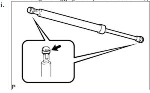
Attach the two stop rings to the luggage compartment door support ASSY.
