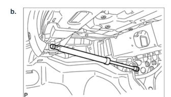
Attach the luggage compartment door support ASSY to the ball joint.
