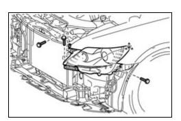
14. REMOVE HEADLIGHT ASSEMBLY LH (w/ Headlight Cleaner System)
