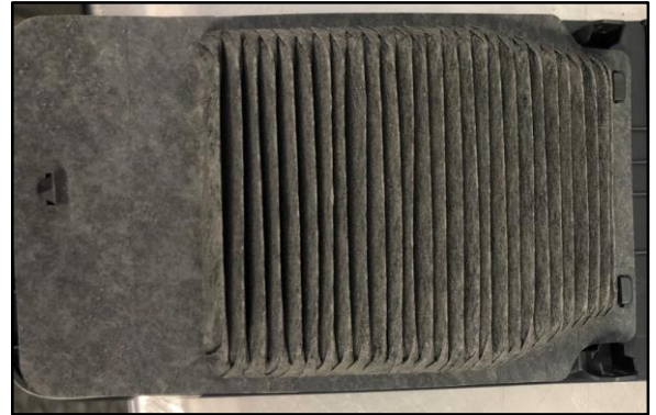
Figure 2. Example of a UX 250h Battery Intake Filter
