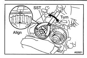
(d) Using SST, align the dot mark on the camshaft timing timing pulley with the timing mark of the No. 4 timing belt cover.
