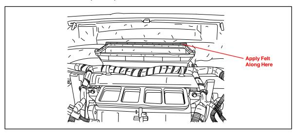
5. Apply foam to the instrument pad HVAC duct as shown in the following illustration.
