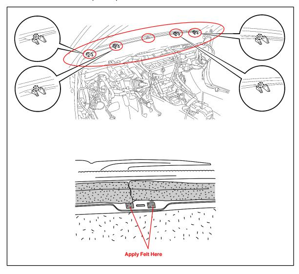
Repair Procedure (Continued) 4. Apply felt along the defroster nozzle lip as shown in the following illustration.
