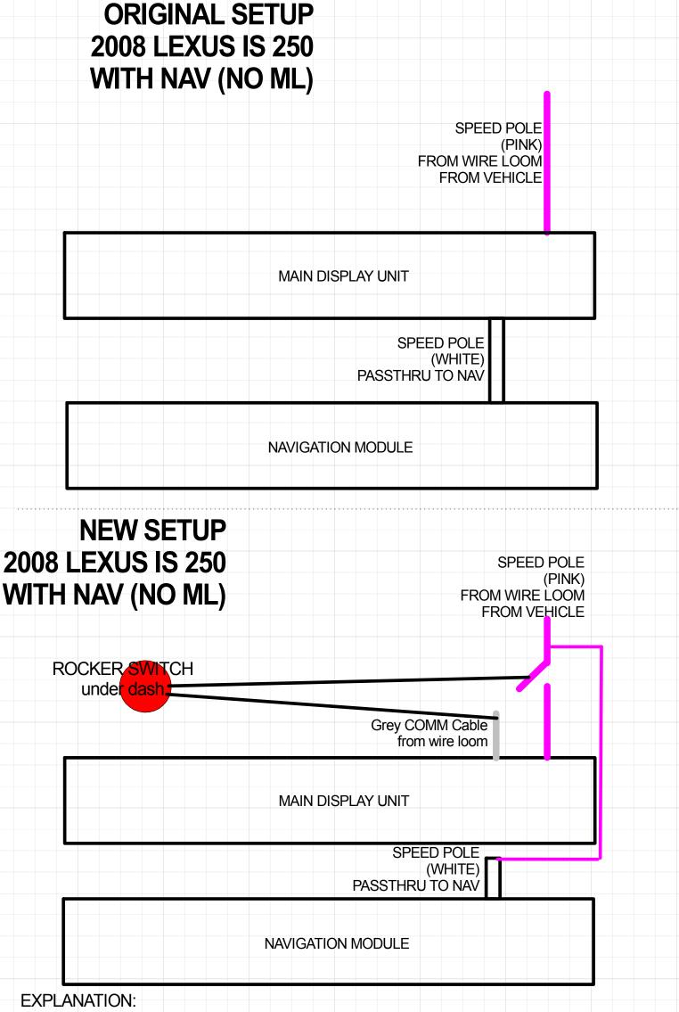
THE MAIN SPEED POLE FROM THE ENGINE HAS TO BE JUMPED TO THE SPEED WIRE THAT GOES FROM THE MAIN DISPLAY TO THE NAV. THE MAIN SPEED WIRE HAS TO BE SWITCHED TO GIVE YOU "FACTORY" MODE OR "HACKED" MODE.
