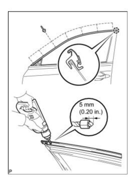
(a) Put a 4 mm (0.16 in.) drill bit into a drill.
