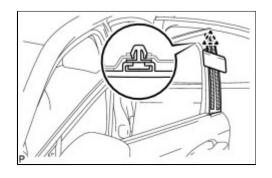
(c) Using a moulding remover, remove the clip and front door rear window frame moulding.
