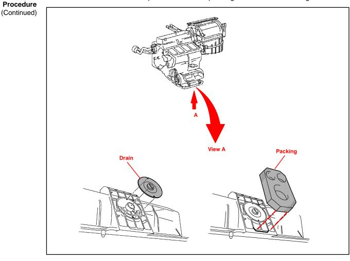
**Repair** 3. Install the NEW HVAC evaporator drain and packing to the air conditioning unit.
