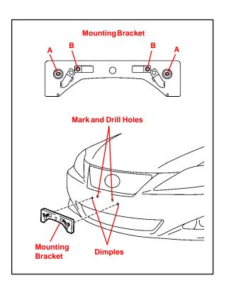
Installation Procedure (Continued) 3. Install the mounting bracket to the front bumper cover at holes "A" using the two supplied self-tapping screws.
