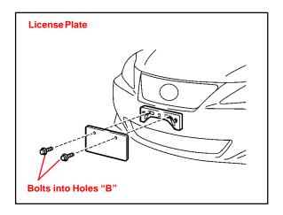
Use bolts of a non–corroding type with the following dimensions to install the front license plate:
