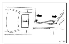
Adjust by loosening the sliding roof installation nuts and readjust the sliding roof to the proper position.
