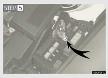
Remove the fuse with the pullout tool.
