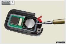
Remove the depleted battery.
