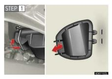
Release the lock and remove the cover.
