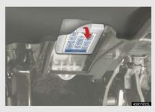
▶ Driver's side instrument panelRemove the lid.
