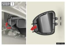
Release the lock and remove the cover.
