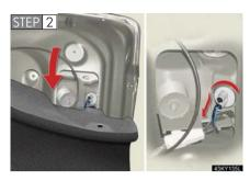
Partly remove the trunk panel cover and turn bulb bases counterclockwise.
