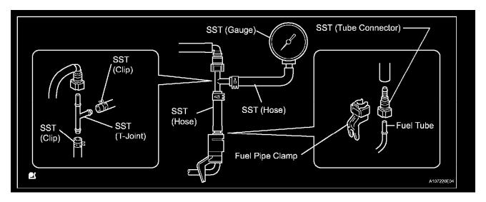
e. Install SST (pressure gauge) as given in the illustration.
