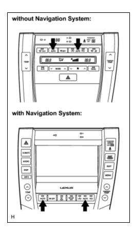
(b) Turn the engine switch on (IG) while pressing the A/C control "AUTO" switch and "R/F" switch simultaneously. Hold both switches until the indicator check screen appears.
