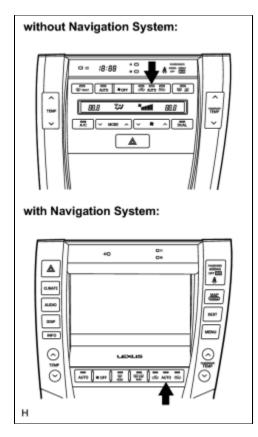
(c) Push the "R/F" switch to perform the actuator check.
