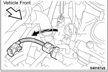
b) Route the sensor harness from behind the heater hose.
