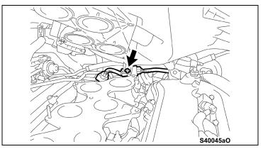
r) Detach the clamp of the SCV position sensor connector from the surge tank.
