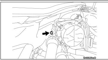
f) Using the supplied box wrench remove the bolt for the water pipe stay.
