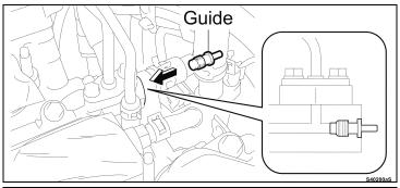
c) Install the guide into the end of the fuel delivery pipe finger tight.
