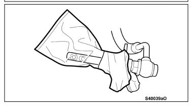
k) Cover the cold start injector to prevent damage.
