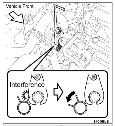
NOTE: It may be necessary to rotate the clamp for the heater hose to allow the wrench to fully seat on the sensor.
