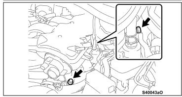
p) Remove the 2 bolts from the side of the air surge tank.
