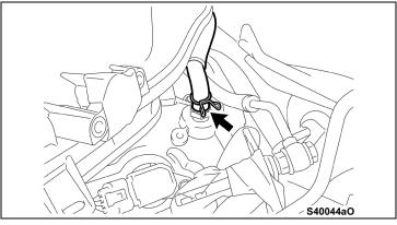
q) Move the surge tank and disconnect the left rear bank ventilation hose.
