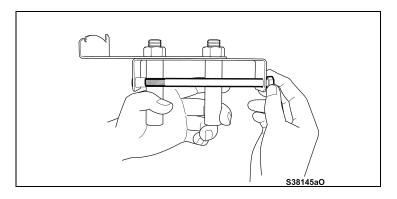
b) Remove the bolt from the supplied GR torque angle plate.
