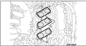
v) Place protective tape over the intake manifold ports to prevent foreign objects from entering.
