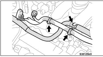
e) Disengage the 2 wire harness clamps and disconnect the No.2 water by-pass hose from the air surge tank.
