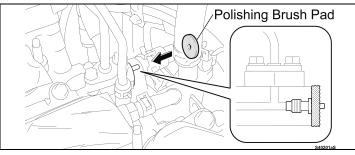
f) Place the NEW polishing pad onto the guide at the end of the fuel delivery pipe.
