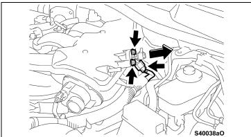
i) Disconnect the cold start injector.
