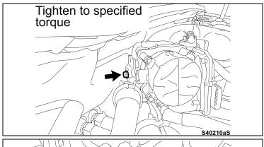
t) Tighten the bolt for the water pipe stay.
