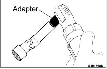
g) Check that the air ratchet will rotate clockwise.
