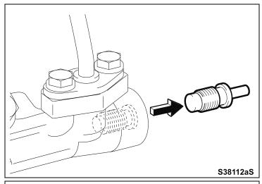
n) Remove the guide from the end of the pipe.
