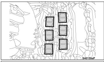
d) Cover the openings with tape to prevent foreign objects from entering the intake ports.
