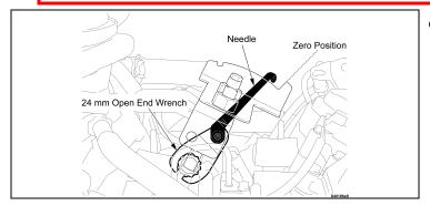
e) Place the 24 mm wrench onto the sensor with the needle as close as possible to the zero position of the torque plate.
