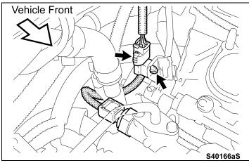
4. REMOVE THE FUEL PRESSURE SENSOR
