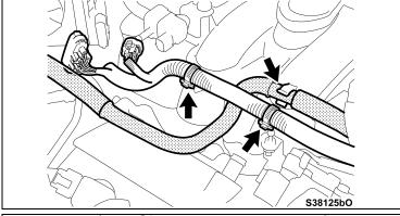
u) Reinstall the No.2 water by-pass hose and reinstall the wire harness clamp.
