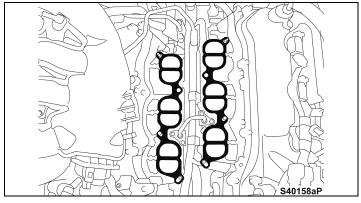
c) Remove and discard the intake manifold gaskets.
