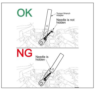
f) Attach the torque wrench adapter to the 24 mm wrench.
