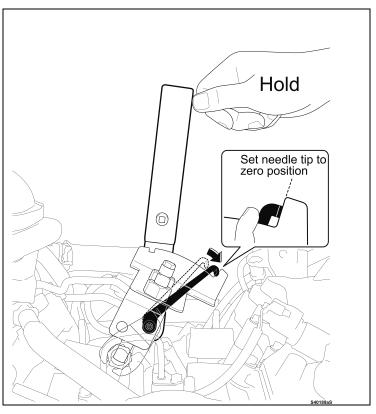
h) While holding the torque adaptor gently move the needle on the 24 mm wrench to the zero position on the plate.
