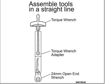
g) Assemble the 24 mm wrench, torque adapter and the supplied torque wrench as shown.
