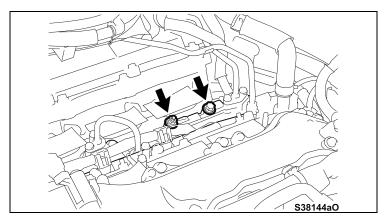
m) Reinstall the bolt and nut for the right fuel delivery pipe.
