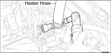
i) Insert the polishing tool behind the heater hose and engage it onto the guide.
