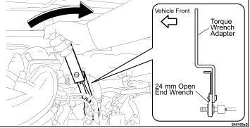
d) Attach the supplied torque wrench adaptor to the 24 mm wrench as shown and loosen the sensor.
