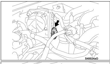
b) Disconnect the throttle body connector.
