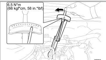
h) Tighten the sensor as shown until the specified torque reading is obtained.
