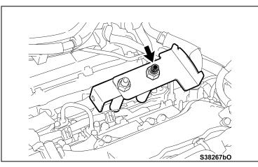
k) Remove the bolt shown and remove the plate.
