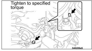
k) Tighten the 2 bolts on the side of the surge tank.
