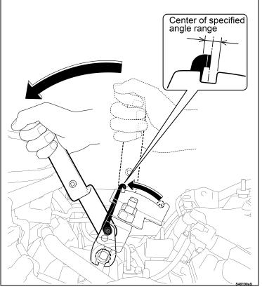
i) Tighten the sensor until the needle tip aligns with the center of the cut out in the plate as shown.
