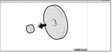
d) Inspect the polishing pad that is contained in the parts kit. Ensure that the center piece of the new pad is removed.
