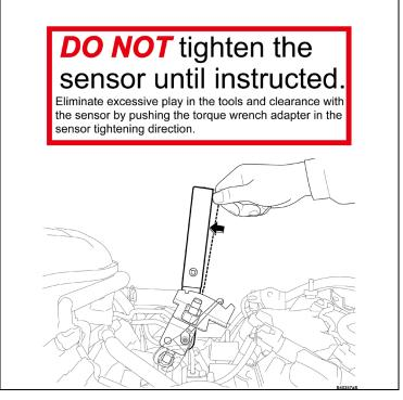
g) Lightly push and hold the torque adapter as shown to eliminate any play but do not rotate the sensor.
