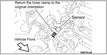
n) Return the clamp for the heater hose to its original position if necessary.
