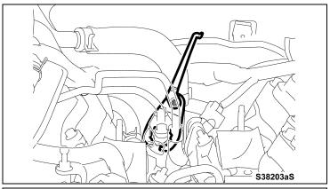
f) Place the 24 mm wrench onto the sensor.
