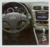
MANUAL OVERRIDE The paddles (left) behind the steering wheel allow the driver to shift gears manually, but the response isn't particularly quick. The IS 250's center console (above) has an MP3 input jack.
