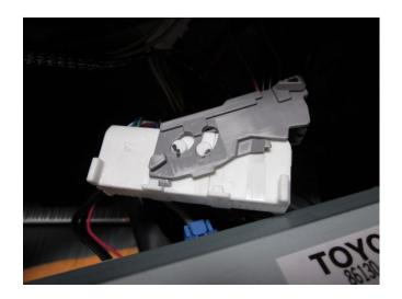
Once the main connector is in one piece with the gray bracket, insert it back to behind the oem head unit
