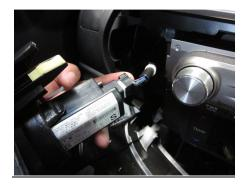
Route the push button switch wire to the side of the radio to your desired location. We chose to place it right under the parking brake lever.
