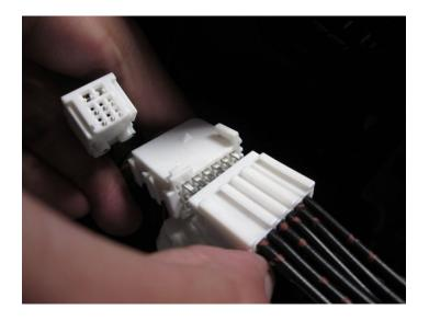
Take the female side of the NT6223 connector and link it back to the main connector, then mount the gray bracket back to the main connector.
