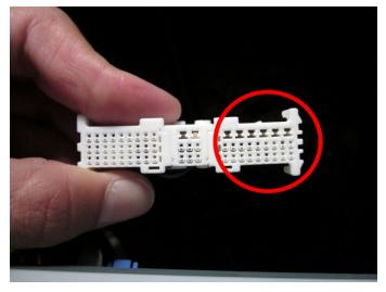
Connect the male side of the NT6223 connector to the female connector which was disconnected from the previous step. Make sure the connection is secure and that none of the pins are exposed on the side.
