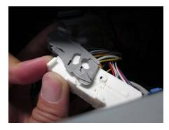
After the gray bracket is removed, the connector should look like this. The right side of the connector is what you need to disconnect from the main connector.
