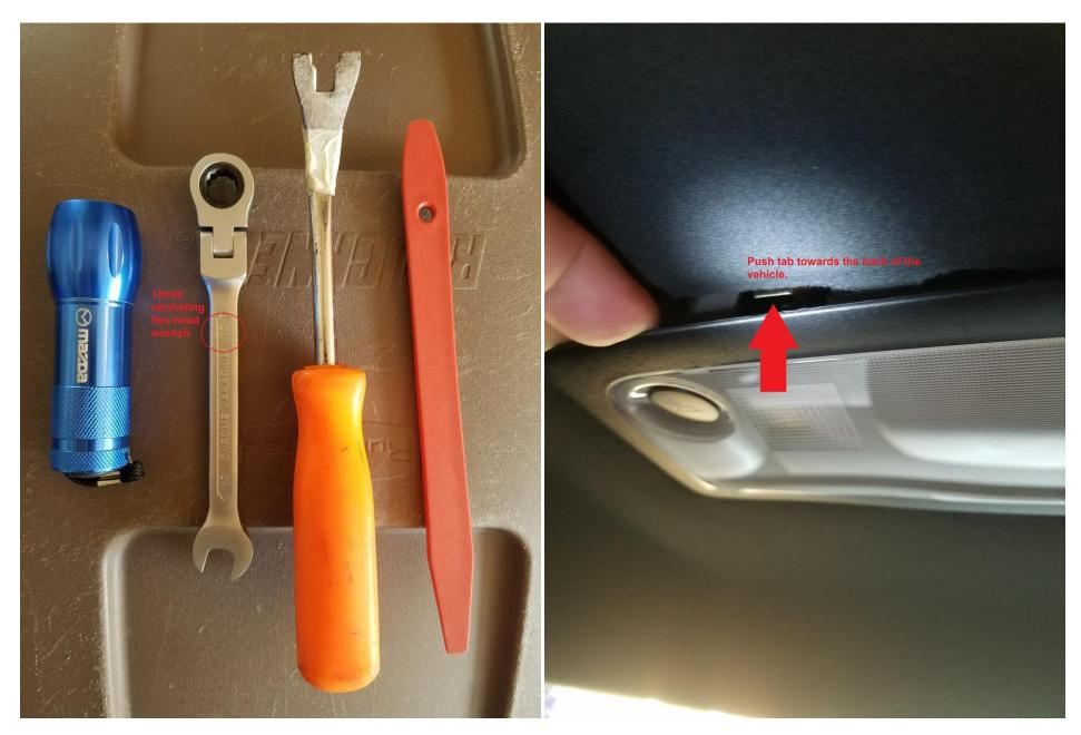
Tools: Flashlight, 10mm ratcheting flex head wrench, metal forked trim tool, composite trim tool. Any flashlight with a 1-1.25 inch head will work...the trim tools don't have to be exactly like the ones above. To ratcheting wrench is a must...or one very similar to it.
