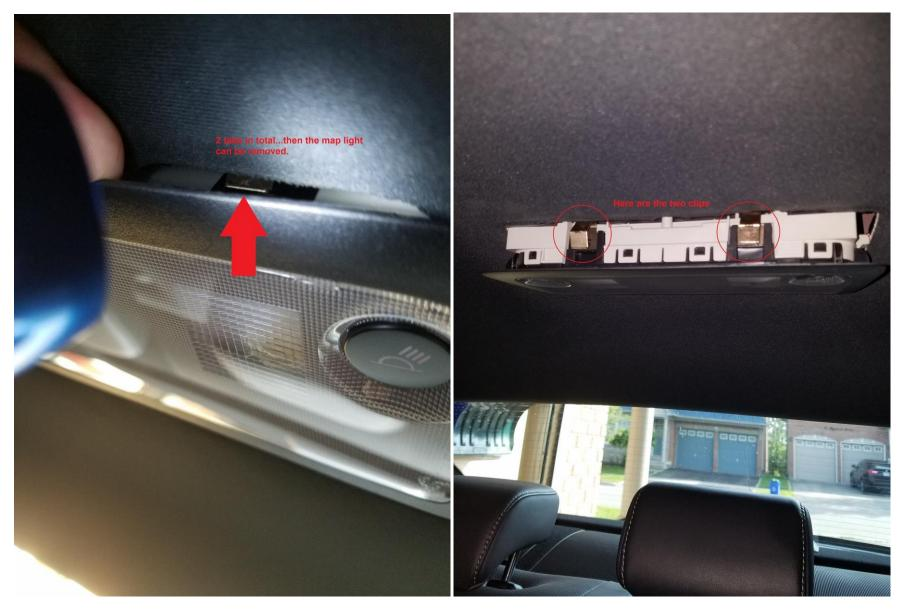
There are two metal tabs to release one side of the map light, which will allow it to be removed. The map light has 4 tabs in total, but releasing the two on the front was the easiest to get the light down.
