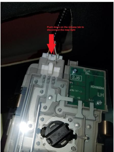
Push down on the plastic tab and pull the connector out.
