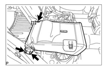
(e) Disengage the guide to remove the rear seatback assembly RH.
