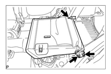
(e) Disengage the guide to remove the rear seatback assembly LH.
