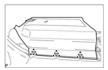
(c) Disengage the 5 fasteners as shown in the illustration.
