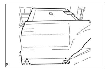
(c) Disengage the 4 fasteners as shown in the illustration.
