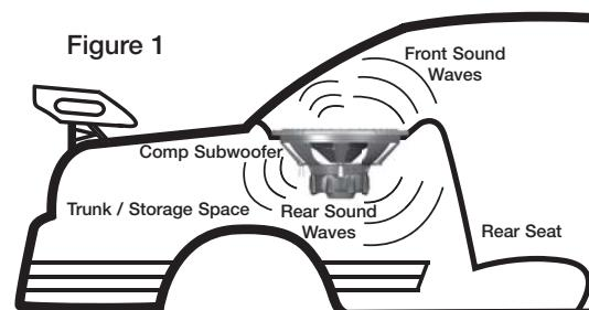
Carefully mount loudspeakers in the trunk space or in other compartments of the vehicle. Pay attention to cable lines, trunk springs, hinges and seat mechanisms that could cause problems with the operation of the vehicle or stereo system. Carefully lay the stereo system cables; pay attention to seat fasteners and other items that could harm the cables.
