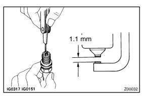
(f) Check the spark plug electrode gap.
