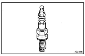
(e) Check the spark plug for thread damage and insulator damage.
