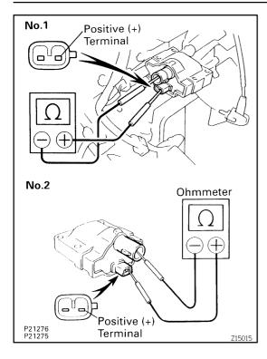
(d) Using an ohmmeter, measure the secondary coil resistance between the positive (+) and high-tension terminals.
