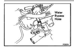
(g) Connect the water bypass hose to the water inlet housing.
