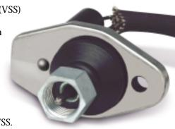
Before powering a digital dashboard, the VSS was used to regulate the cruise control and control transmission shifts. Now, depending upon vehicle equipment, the VSS may influence or control more systems than any other single sensor.
