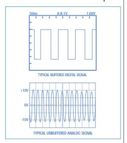
In some cases, you can even count VSS cycles with a DVOM. Use the analog bar because the digital display usually won't be fast enough or accurate enough to give reliable readings.
