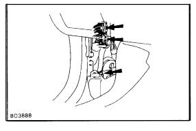
(b) Disconnect three connectors as shown.
