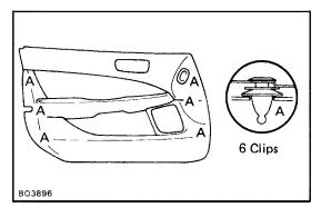
(c) Insert the screwdriver between the panel and the trim and remove the clips.
