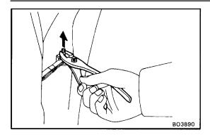
(b) Using the pliers, push out the arm pin and disconnect the door check from body.
