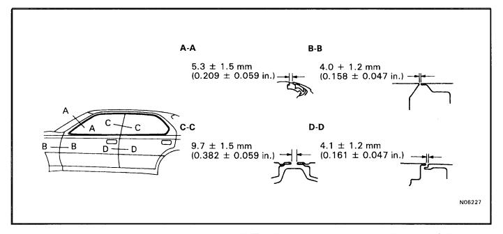
HINT: Adjust the door panel according to the following method.
