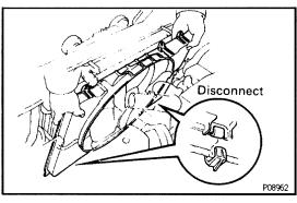
(b) Disconnect the lower sides of the No.1 fan shroud from the 2 hooks of the radiator, and remove the radiator.
