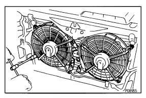
(e) Remove the 2 bolts and cooling fan. Remove the 2 cooling fans.
