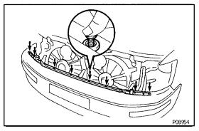
INSTALL UPPER BUMPER RETAINER Install the bumper retainer with the 8 clips.
