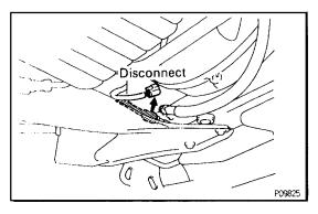
(c) Disconnect the ECT switch connector.
