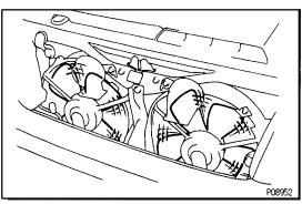
(d) Check that the cooling fans rotate. If not, check the engine main relay, cooling fan relay, cooling fan, fuses, and check for short circuit between the cooling fan relay and ECT switch.
