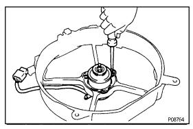
(b) Remove the 3 screws and fan motor.
