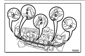
9. REMOVE UPPER FRONT BUMPER REINFORCEMENT Remove the 10 bolts and front bumper reinforcement.
