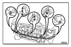
3. **INSTALL UPPER FRONT BUMPER REINFORCEMENT** Install the front bumper reinforcement with the 10 bolts.
