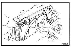
(b) Install the No.1 fan shroud with the 3 bolts.
