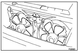
(b) Check that the cooling fans stop. If not, check the cooling fan relay and ECT switch, and check for a separated connector or severed wire between the cooling fan relay and ECT switch.
