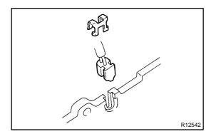
(e) Right wheel: Connect the pad wear indicator to the inner pads, and install a new clip.
