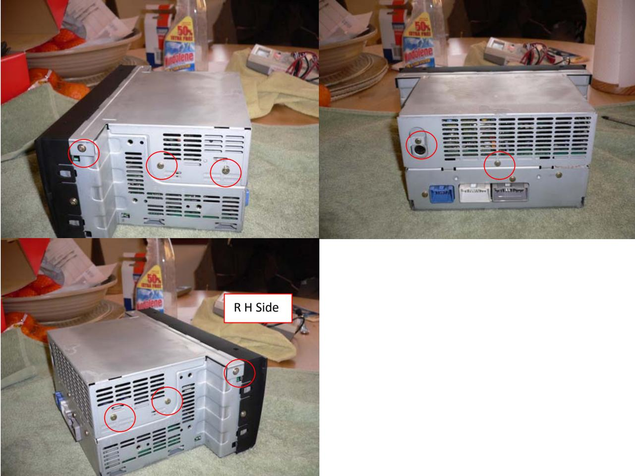
1. Identify and remove the 8 screws circled red shown in the photographs above and carefully liftoff the top of the stereo.
