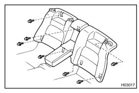
(c) Remove the 7 bolts, then raise the seatback assembly upward to remove the seatback assembly.
