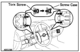
(e) Pull the wheel pad out from the steering wheel and disconnect the airbag connector.
