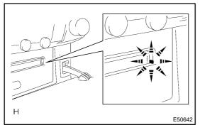
(c) While holding the "UP" and "DISC" switches, turn the ignition switch to the ACC position.
