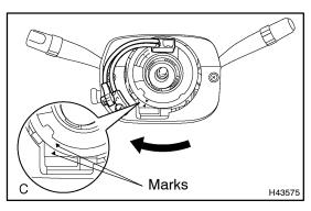
(d) Rotate the spiral cable sub-assy clockwise approximately 2.5 turns to align the marks.
