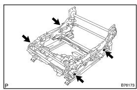
**26. REMOVE POWER RECLINING ADJUSTER ASSY** Using a T40 torx<sup>®</sup> socket wrench, remove the 4 torx<sup>®</sup> screws and the power reclining adjuster.
