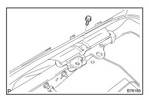
(e) Install the seatback cover hook with the bolt. Torque: 5.2 N⋅m (54 kgf⋅cm, 47 in.·lbf)
