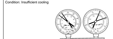
NOTE: These gauge indications are shown when the refrigeration system has been opened and the refrigerant charged without vacuum purging.
