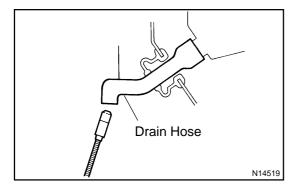
(b) Bring the gas leak detector close to the drain hose before performing the test.
