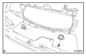
**17. REMOVE NO. 1 METER HOOD RETAINER** Remove the screw and No. 1 meter hood retainer.
