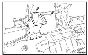
8. REMOVE NO. 2 HEATER TO REGISTER DUCT
