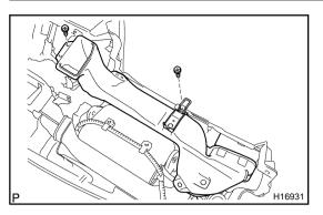
9. REMOVE NO. 4 HEATER TO REGISTER DUCT
