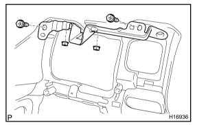
REMOVE NO. 4 FINISH PANEL MOUNTING BRACKET Remove the 2 screws and No. 4 finish panel mounting bracket.
