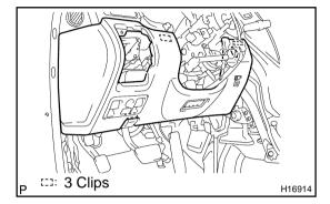
(c) Using a screwdriver, remove the No. 1 safety pad. HINT:
