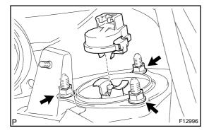
(c) Turn the actuator counterclockwise to 40° and remove it upward.
