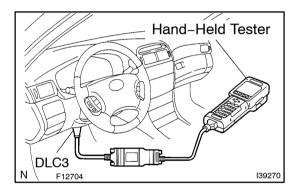
(b) Connect the hand-held tester to the DLC3, then turn the ignition switch to the ON position.
