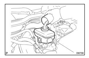
FILL RESERVOIR WITH BRAKE FLUID 1. Fluid: SAE J1703 or FMVSS No. 116 DOT3
