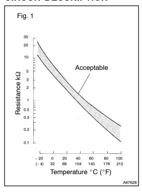
A thermistor is built in the Engine Coolant Temperature (ECT) sensor and changes the resistance value according to the engine coolant temperature.
