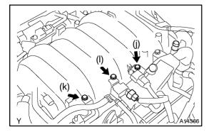
(j) Install the V-bank cover bracket No. 3 with bolt.
