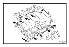
(b) Install the upper and lower intake manifolds assembly with the 6 bolts and 4 nuts.
