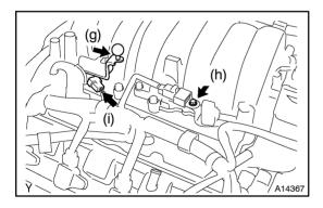
(g) Install the V-bank cover bracket No. 4 with bolt.
