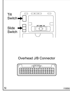
(a) Remove the overhead J/B assembly.
