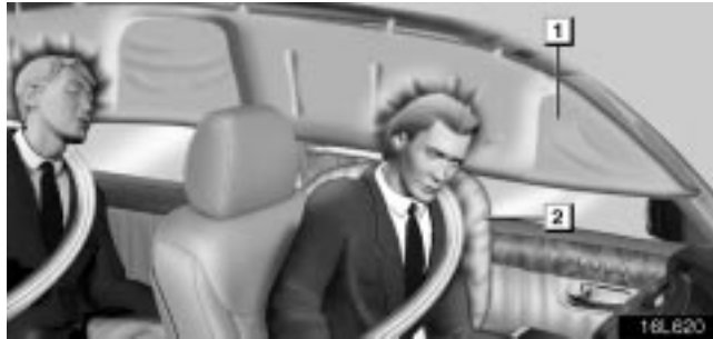
► 1 Curtain shield airbag 2 Side airbag
