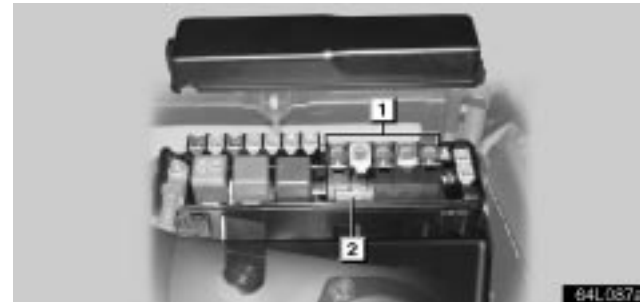
► Engine compartment 1 Spare fuses 2 Pull-out tool
