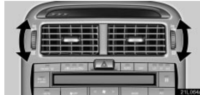
The center vents may be opened or closed as shown.
