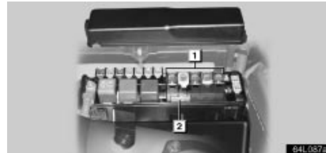
► Engine compartment 1 Spare fuses 2 Pull-out tool
