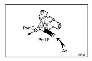
(a) Check that air flows with difficulty from ports F to E.OK: Air flows with difficulty from ports F to E.
