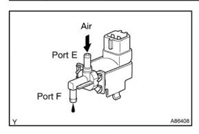
(a) Check that the air flows with difficulty from ports E to F.OK: Air flows with difficulty from ports E to F
