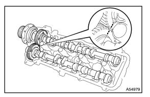
(a) Apply MP grease to the thrust portions of the camshafts.
