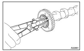
(c) Using snap ring pliers, remove the snap ring.
