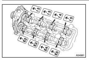
Install the front bearing cap.
