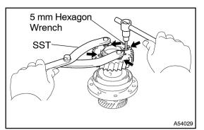
(j) Using SST and a 5 mm hexagon wrench, remove the 4 bolts, drive gear and oil seal.
