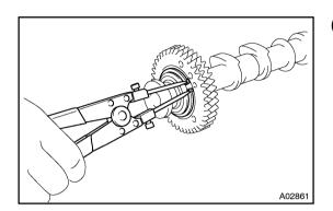
(b) Using snap ring pliers, install the snap ring.
