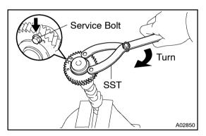
(b) Using SST, turn the sub gear clockwise and remove the service bolt.
