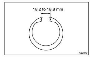
(e) Using vernier calipers, measure the gap distance of the gear spring.
