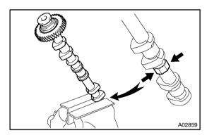
(c) Mount the hexagonal portion of the camshaft in a vise. **NOTICE:**
