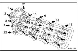
Uniformly tighten the 22 bearing cap bolts in several (m) steps, in the order shown in the illustration. Torque: 7.5 N·m (76 kgf·cm, 66 in.·lbf) for bolt C
